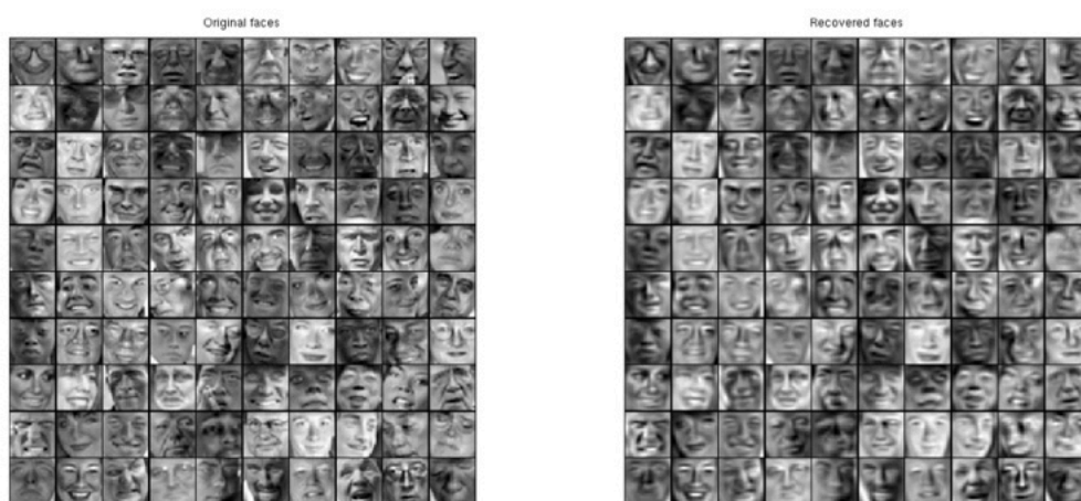
Figure 9: Original images of faces and ones reconstructed from only the top 100 principal components.
